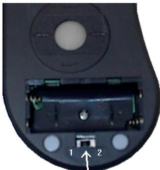
**Figure 1: The bottom of the mouse with an open battery compartment**
