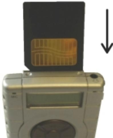
**Figure 8: Inserting the memory card**
