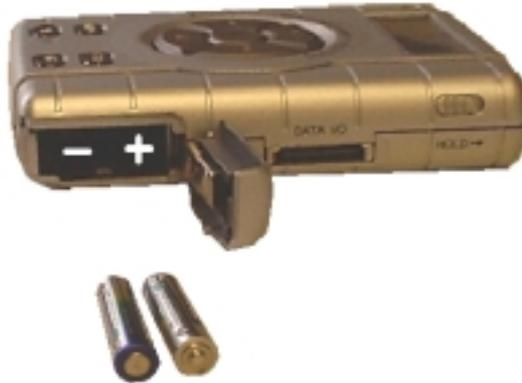
**Figure 7: Inserting the batteries**
