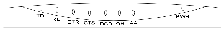
Figure 1: The indicators on the front of the modem
