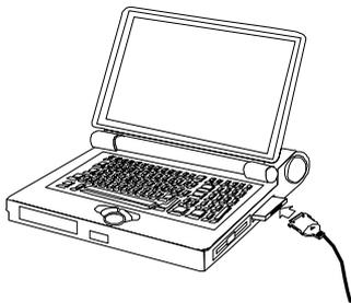
Figure 2: Attaching the modem cable
